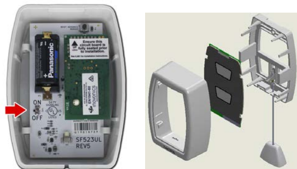
Figure 3 - SF523UL Battery On/Off Switch and Assembly
