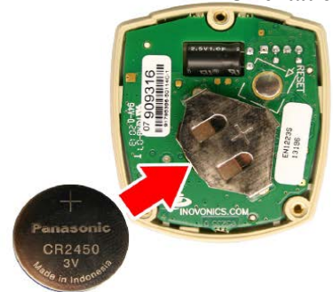
Figure 9 - SF501ES Battery Orientation
