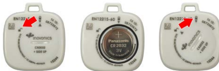
Figure 6 - SF503UL and SF504ES Battery Replacement
