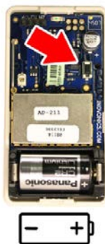
Figure 13 - SF502ES Battery Orientation
