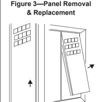
Panel Removal: First remove the self-tapping metal screws located in the top U-channel just above each panel. Then lift up on panel to clear bottom channel. After removal, adequate space is available to grasp and remove the remaining panels.
