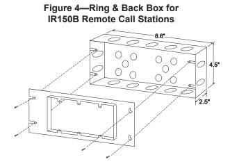
Install ring with panel mounting holes at top and bottom, as shown.
