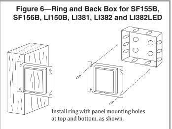
**LI382LED Corridor Zone Light:** Install standard one- or two-gang box with one- or two-gang ring as shown in *Figure 6* for each corridor light in system. Ring and back box must be UL® approved. Minimum clearance from live parts of station to dead metal parts to be not less than 0.5".
