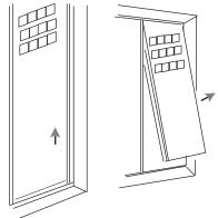
Panel Removal: First remove the self-tapping metal screws located in the top U-channel just above each panel. Then lift up on panel to clear bottom channel. After removal, adequate space is available to grasp and remove the remaining panels.
