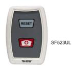
( The SF523UL Room Station is a wireless, surface-mountable station that includes a call button, an optional plastic pull cord, an LED for call indication, and a reset button. The SF523UL is provided with three interchangeable label inserts for different uses such as "Help," "Assist/Check-In," and "Emergency" calls. The SF523UL features a battery on/off switch to preserve the life of the battery when shipped.
