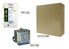
**The IH151NK Power & Control Kit** provides power and control for two states (steady/ routine and flashing/emergency) to dome lights when used with an NC50xES-series remote receiver. The kit includes a PK152 Power & Control Unit and an SS106 Class 2 Transformer installed in an IH151N junction box. The PK152 uses pigtail connections. Knockouts are included on all sides (except the lid) to allow the connection of electrical conduit from any direction.
