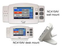
The NC415AV Master Station provides audible and visual call indication without intercom communications. Its color LCD touch screen displays 3 calls at once, with scrolling for additional calls. The NC415AV may be desk mounted or wall mounted. An LI484P5 corridor light may be connected directly to the master station as a zone light. Wiring is simple CAT5e or better. Includes audio/visual license.
