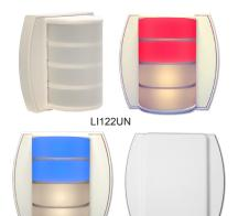
The LI122UN Room Controller with Dome Light provides 6 connection points for patient stations, 2-button pull-cord stations, and a duty station; plus visual indication of calls via slide switches to manually select the two dome colors as White/Red or White/Blue and tone of the White color as warm White or cool White. The PM120 Room Controller provides the same 6 connection points in locations where a corridor dome light is not needed.
