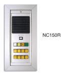
**The NC150R Master Station Panel** is flush wall mounted and constructed of extruded aluminum. The NC150R includes the speaker, control module, amplifier, frame and 8 lamp/buttons to accommodate up to 8 areas of rescue. (Larger masters are available on a special-order basis.) Lamp/buttons have removable lenses for easy identification.
