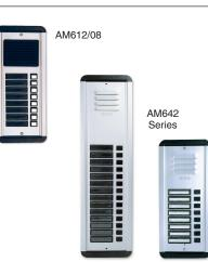
AM612-series Vandal-Resistant Entrance Panels and AM642-series Entrance Panels are available in a 4.75" × 11.25" (119 mm × 282 mm) version that accommodates up to 8 buttons, and a 4.75" × 17.25" (119 mm × 432 mm) version for 10–16 buttons plus name holders. Name holders are constructed of black, flame-retardant polycarbonate plastic with clear plastic windows. Panels are constructed of anodized extruded aluminum with black plastic end caps.
