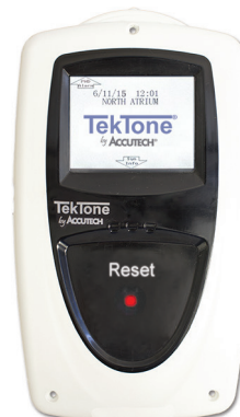
annunciator with touchscreen and reset button
