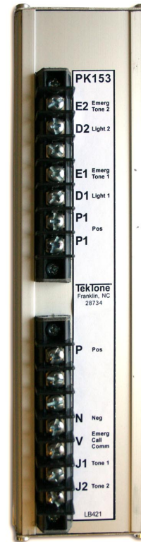
PK153 Third Priority Control Unit
